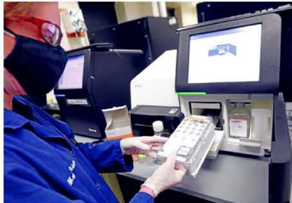
Amanda Maegli, research specialist at the DNA sequencing lab at the UW-Madison Biotechnology Center, loads a cartridge with DNA samples into a DNA sequencer.
